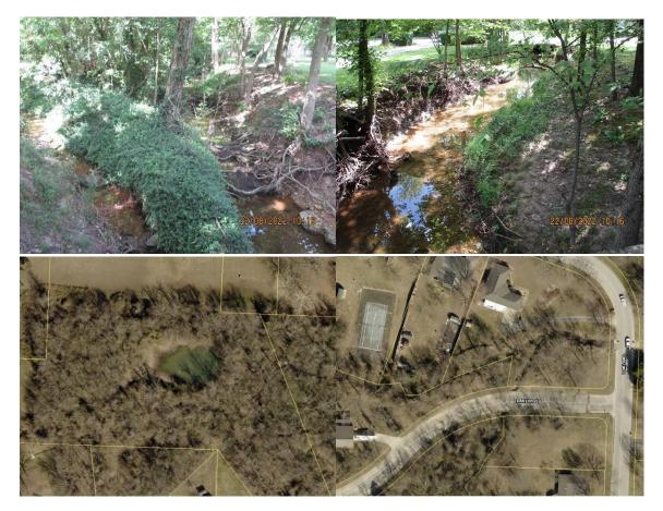
PROJECT DESCRIPTION: The goal of this project is to widen the creek on the northside of Lakewood Drive to allow more flow downstream to reduce flooding on the southside of Lakewood Drive. The second goal is to create a regional detention basin out of the pond to reduce the peak flow from Tracker and Killingsworth Ave. The City Engineer has met with MS4 and the Public Works Director to review this future project.
