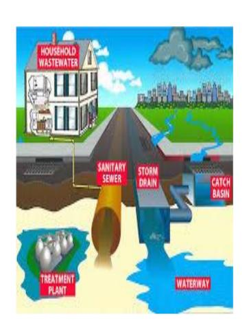
A conveyance or system of conveyances (including roads with drainage systems, municipal streets, catch basins, curbs, gutters, ditches, manmade channels, or storm drains) owned or operated by the United States, a State, city, town, county, district, association, or other public body...that discharges to waters of the United States or waters of the State that is designed or used for collecting or conveying stormwater.
